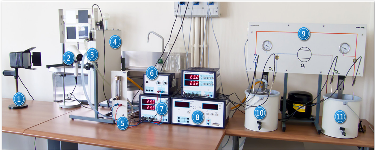
Picture 1. Heat pump – solar collector experimental set-up: 1 – halogen lamp; 2 – hair-dryer; 3 – thermocouple probe; 4 – solar collector; 5 – water pump with flow-metre; 6 – water pump power supply; 7 – digital thermometer; 8 – electrical energy, power and time metre; 9 – heat pump; 10 – heat exchanger and evaporator reservoir; 11 – reservoir with condenser.
