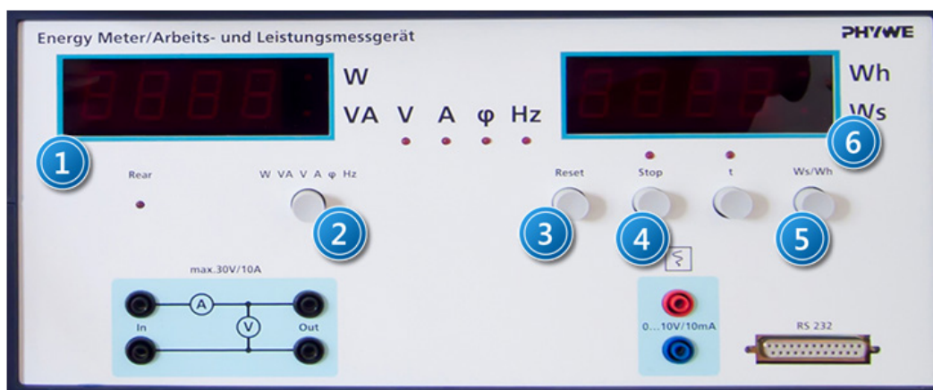
Picture 5. Electrical energy, power and time meter: 1 – power display; 2 – voltmeter function selector; 3 – “RESET” button; 4 – “STOP” button; 5 – button to select energy units; 6 – displays electricity consumed by the pump.
